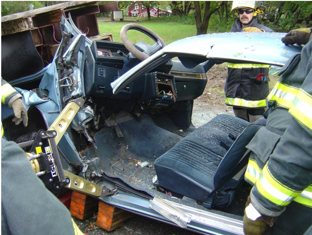
Modified Dash Roll during 40-hour program Swansea, MA FD: Sedan vs. straight truck.
