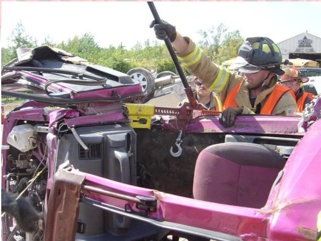
Performing Modified Dash Roll with Hi-Lift Jack and Jack Mate: Vehicle on side.
